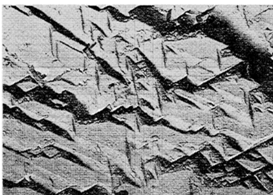
e) The silver(100) surface electrolytically polished in a mixing solution of potassium cyanide and potassium ferrocyanide ( \times 3500 ).
